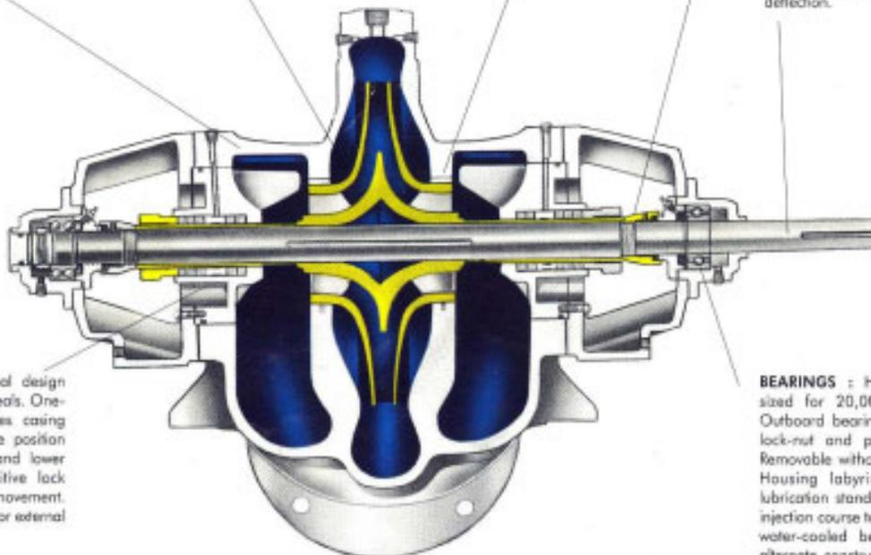
**STUFFING BOX** : Universal design for packing or mechanical seals. One-piece construction eliminates casing split from shaft seal. Single position mounting between upper and lower case halves provides positive lock against rotation and lateral movement. Tapped connection provides for external fluid injection.
