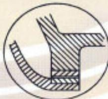
**CASING WEAR RINGS** : Straight type, renewable. Pinned to lower-half casing to provide lock against rotation.
