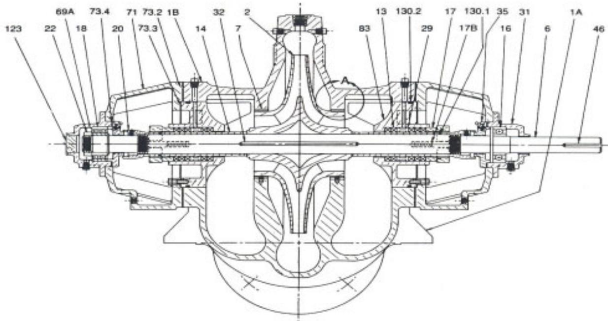
Fig. 1 - Cross Sectional Drawing of Horizontal Split Case Pump Type AD
